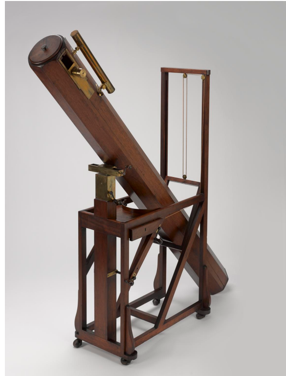
Reflecting telescope made by William Herschel, circa 1783-85, © Science Museum, London, Inv. No. 1876-1000
